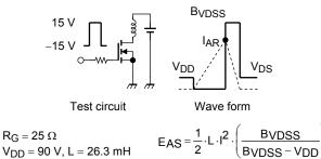
$$V_{DD} = 90 \text{ V, L} = 26.3 \text{ mH}$$
